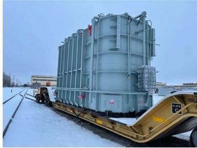
Main power transformer loaded for rail transport
